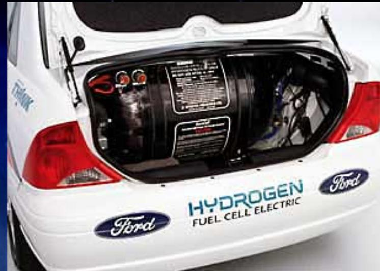
Ford Focus Hybrid Fuel Cell Vehicle combines a high voltage battery with the hydrogen-powered fuel cell engine to help increase performance and efficiency while still providing zero emissions.
